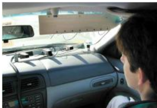
Fig. 3 Array of microphone set up in car .
